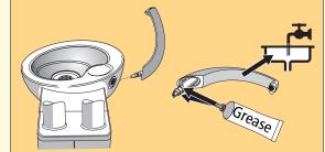
applicable, hydrocolloid adapter and grease O-rings
