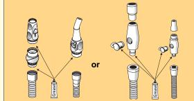
Separate suction handpieces at joint; clean and grease points of separation
